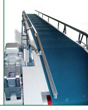
Motorized belts conveyor may have direct motorization (keyed on shaft) or return motorization means by sprocket and chain or pulleys and belts. May have various type of motorization: in terminal part, central part, arc solution ecc...
