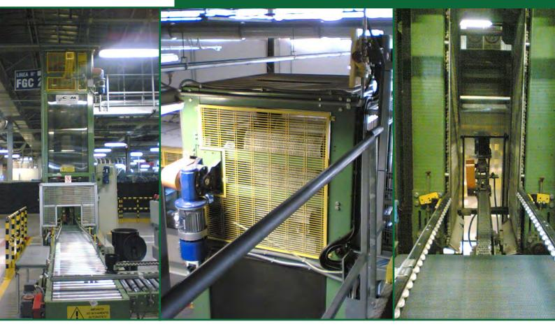
Opposite shelves elevators allow to raise or lower products flow in a factory for improve the internal logistics. It's a continuous movement conveyor that raise or lower one or more product in the same time. The machinery can be formed by painted steel, stainless stell and aluminium.
