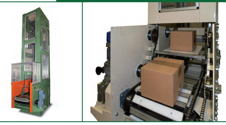
Jointed movable shelves elevator lifters allow to raise or lower products flow in a factory for improve the internal logistics.
