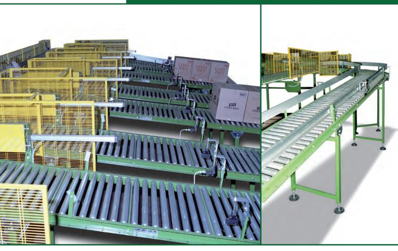
Idle roller conveyors can have roller's diameter and step different type depending the handling product type, from minimum Ø30 mm to maximum Ø60 mm.
