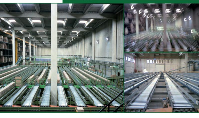
Storage conveyors can have roller's diameter and step different type depending the handling product type, from minimum Ø32 mm to maximum Ø50 mm.
