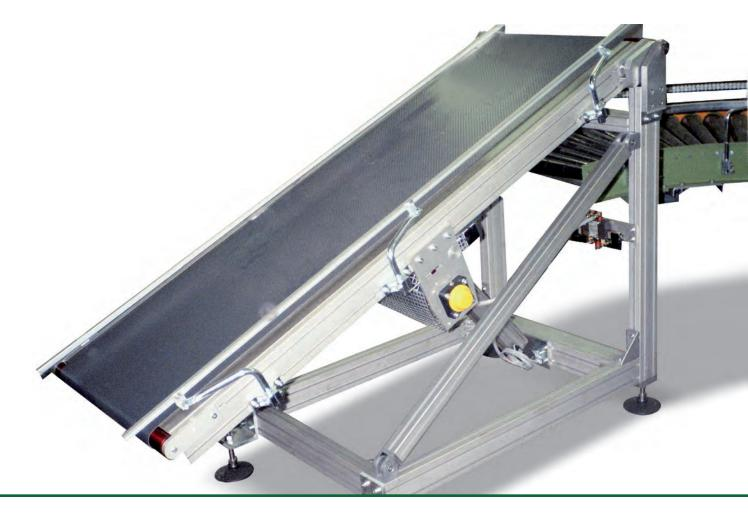
Limited traverse system for conveyors allow to join product flow from different level to the same level or product flow from the same level to different level.
