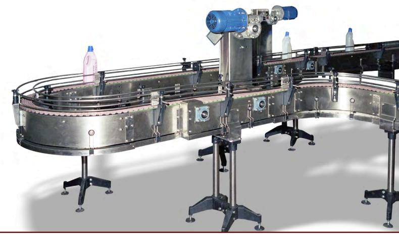
Table-top conveyors width are fixed ad there are choices in relation of handled product type (89,114 mm). Table-top conveyors may have direct motorization (keyed on shaft) or return motorization means by sprocket and chain or pulleys and belts. May have various type of motorization: in terminal part, central part, arc solution ecc...
