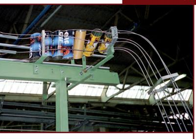
Twist are conveyor link, made by rod stainless steel with different diameter. They can rotate product clockwise or counterclockwise of 90° or 180°.
