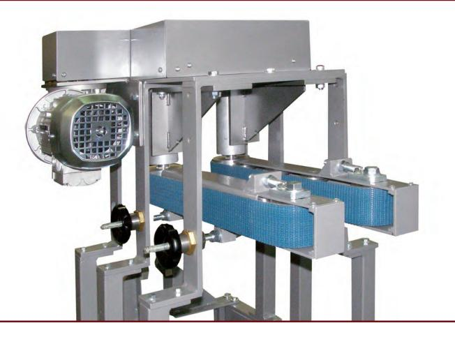
Double belt spacers are component able to pace flow product come from other conveyor. A case for this application, for example, is a machinery that needs a distance between product and other product. Motorized belts conveyor may have direct motorization (keyed on shaft) or return motorization means by pulleys and belts.
