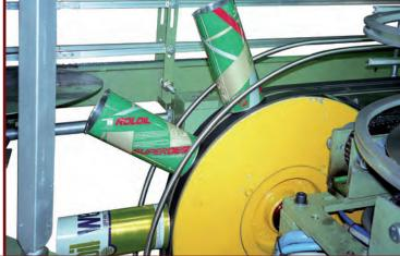
Magnetic lifters allow to raise or lower products flow in a factory for improve the internal logistics. It's a continuous movement conveyor that raise or lower one or more product in the same time. The machinery can be formed by painted steel, stainless stell and aluminium.
