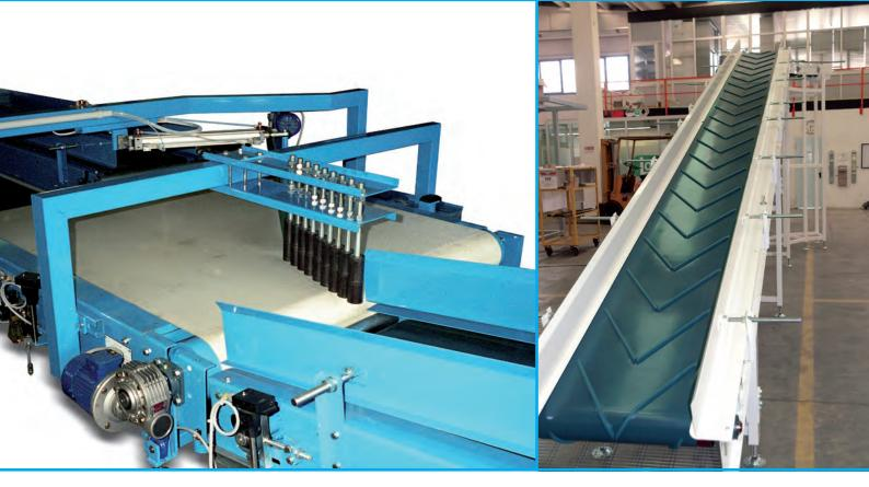
Motorized belts conveyor may have direct motorization (keyed on shaft) or return motorization means by sprocket and chain or pulleys and belts. May have various type of motorization: in terminal part, central part, arc solution ecc.
