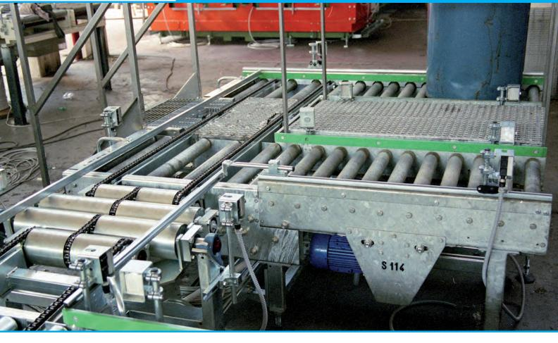
Idle roller conveyors can have roller's diameter and step different type depending the handling product type, from minimum Ø50 mm to maximum Ø76 mm.
