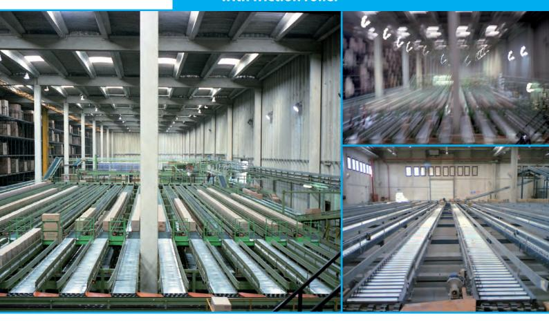
Storage conveyors can have roller's diameter and step different type depending the handling product type, from minimum Ø50 mm to maximum Ø60 mm.
