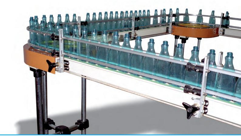
Cable conveyors are suitable to move tins with and without bottom.
