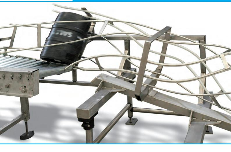
Twist are conveyor link, made by rod stainless steel with different diameter. They can rotate product clockwise or counterclockwise of 90° or 180°.
