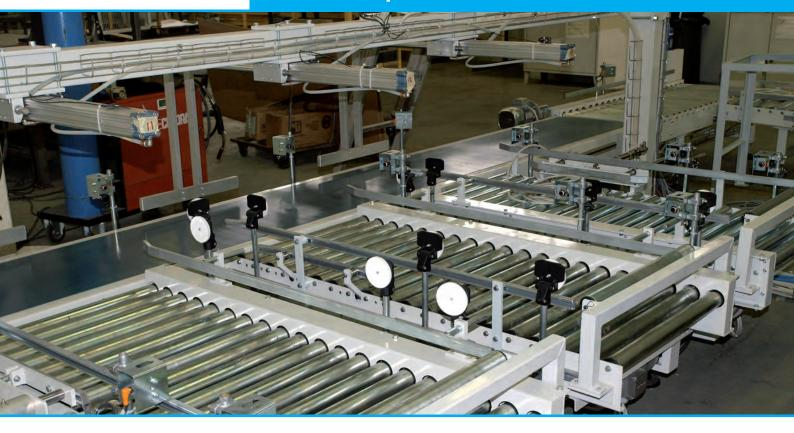
Transfer system can be actuate electromechanically or elettropneumatically. It's function is to translate laterally (90°) the total or partial product flow incoming from other line.
