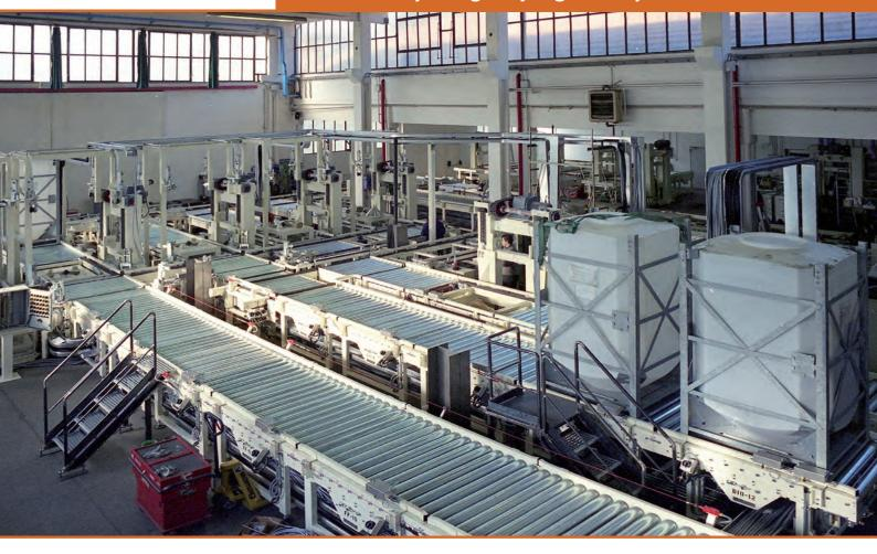
Idle roller conveyors can have roller's diameter and step different type depending the handling product type, from minimum Ø76 mm to maximum Ø105 mm.
