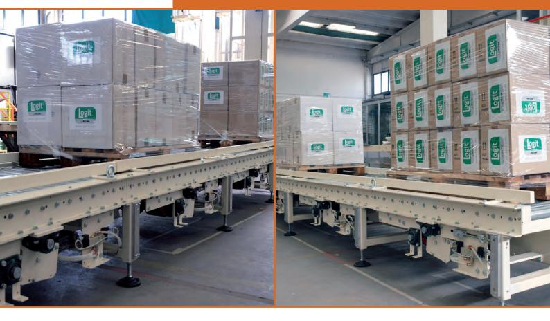
"Acupallet" system meets the requirement to accumulate pallets in a "step by step" modality until 10 stations all operated by a single motor.
