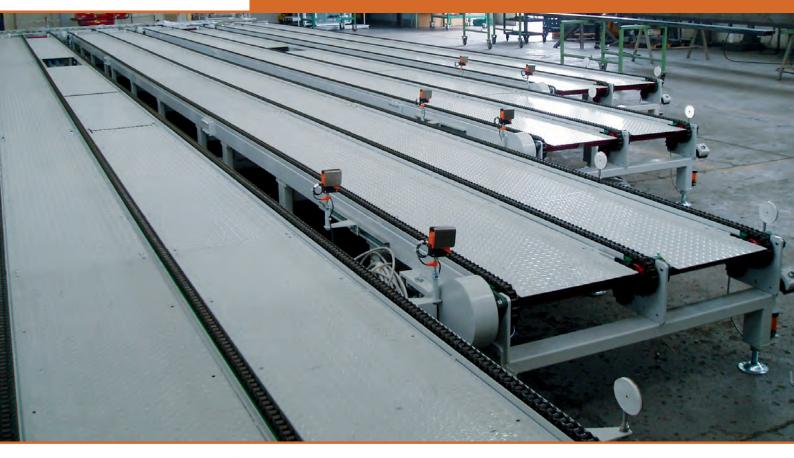
Chain conveyors can have different chain step type, depending the handling product type, from minimum  $\frac{1}{2}$  inch to maximum 1 inch double.
