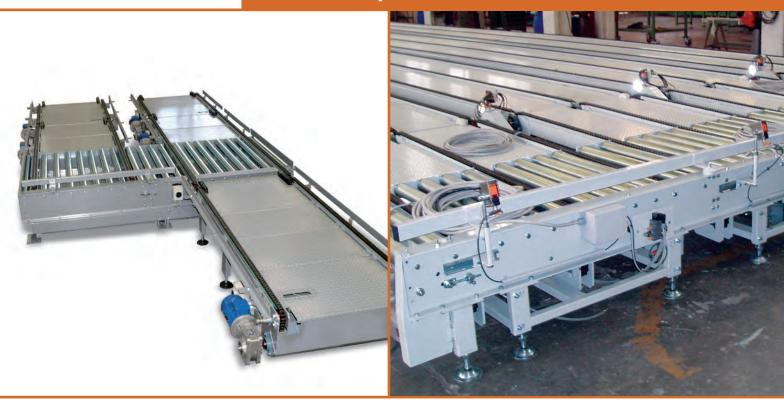
Transfer system can be actuate electromechanically or elettropneumatically. It's function is to translate laterally (90°) the total or partial product flow incoming from other line.
