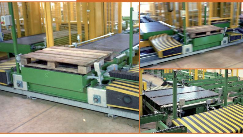
Pallets connecting shuttles use is to connect more conveyors line (for example the exit of palletising machines) in the same gatherer (for example winding pallet line) without change the direction of product. Kinematic motion develops by chain or belt in relation of handled product type and flow product.
