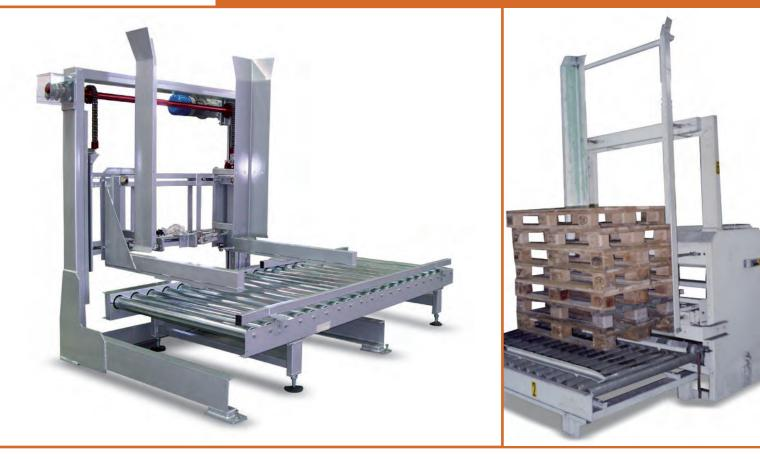
This machinery use is to piling up and unpiling empty pallets for example to serve palletising machines. Kinematic motion for take pallet can be done by fork or lateral arms or levers in relation of handled product type and flow product.
