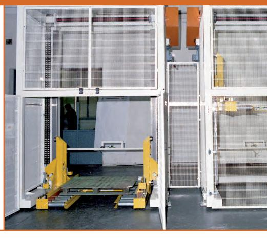
Platform elevator allow to raise or lower products flow in a factory for improve the internal logistics. It's an alternating movement conveyor that raise or lower one or more product in the same time. The machinery can be formed by painted steel, stainless stell and aluminium.
